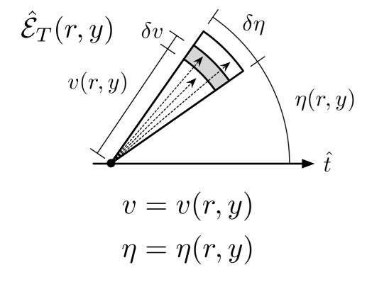
$$\mathcal{E}_T(r,y)|N\rangle = \sum_{i \in N} m_i^{\perp} \delta(r-r_i) \delta(y-y_i)|N\rangle$$
