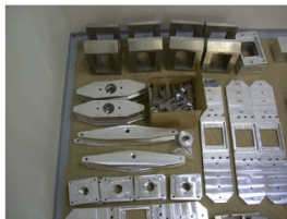
Figure: Roman Pot mechanical parts at machining company in Prague
