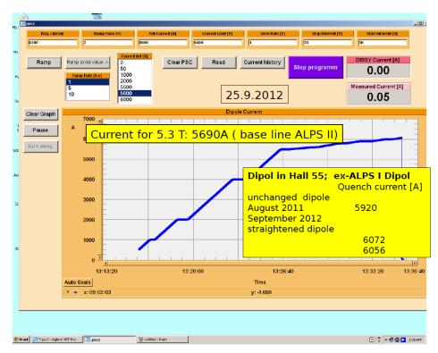
> The straightening procedure for the HERA dipoles has been revised. A simpler and more robust method will be tested soon.
