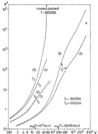
Influence of the structure factor  $S(q)$  on the normalized electrical conductivity  $\sigma^*$ . Dotted line: Coulomb potential for (1)  $S(q) = 1$  and (2)  $S(q)$  in Debye approximation. Full line: Hellmann potential for (3,4)  $S(q) = 1$  and (5,6)  $S(q)$  in mean spherical approximation (MSA).  $x$  - experimental value for cesium at the melting point. The Hellmann potential is recently used to describe the transport coefficients of aluminum.
