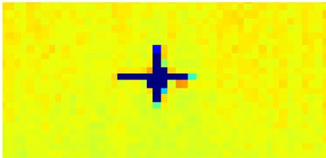
Zoom of spot detail showing diffraction 'cross' and some scatter
