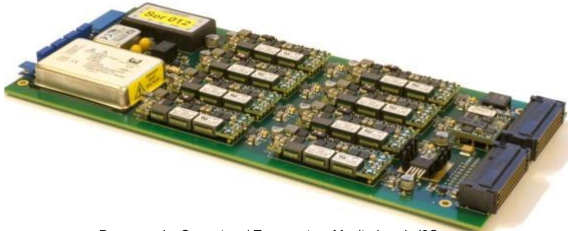
Power card – Current and Temperature Monitoring via i2C
