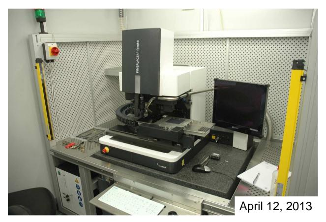
Installed: Femto Flip-Chip Bonder at FEC lab Commissioning in progress
