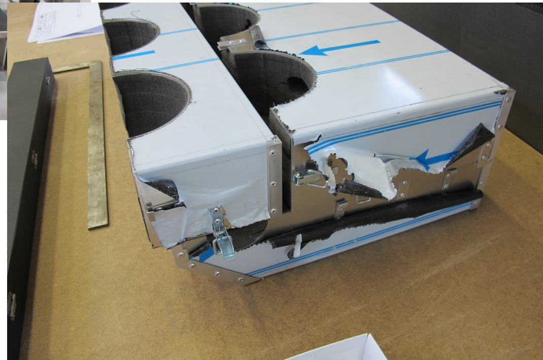
Foam Isolation for the LEWA Pumps
