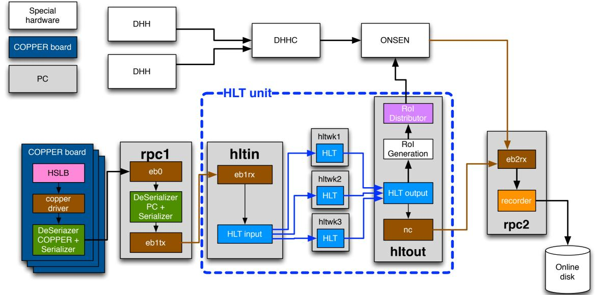
Dummy data come from HSLBs on 3 COPPERs. Dummy Rol data are sent to ONSEN.
