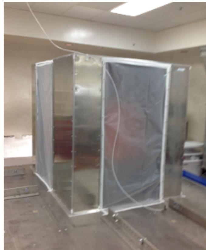
Shield with veto monolith blank and prototype cryostat
