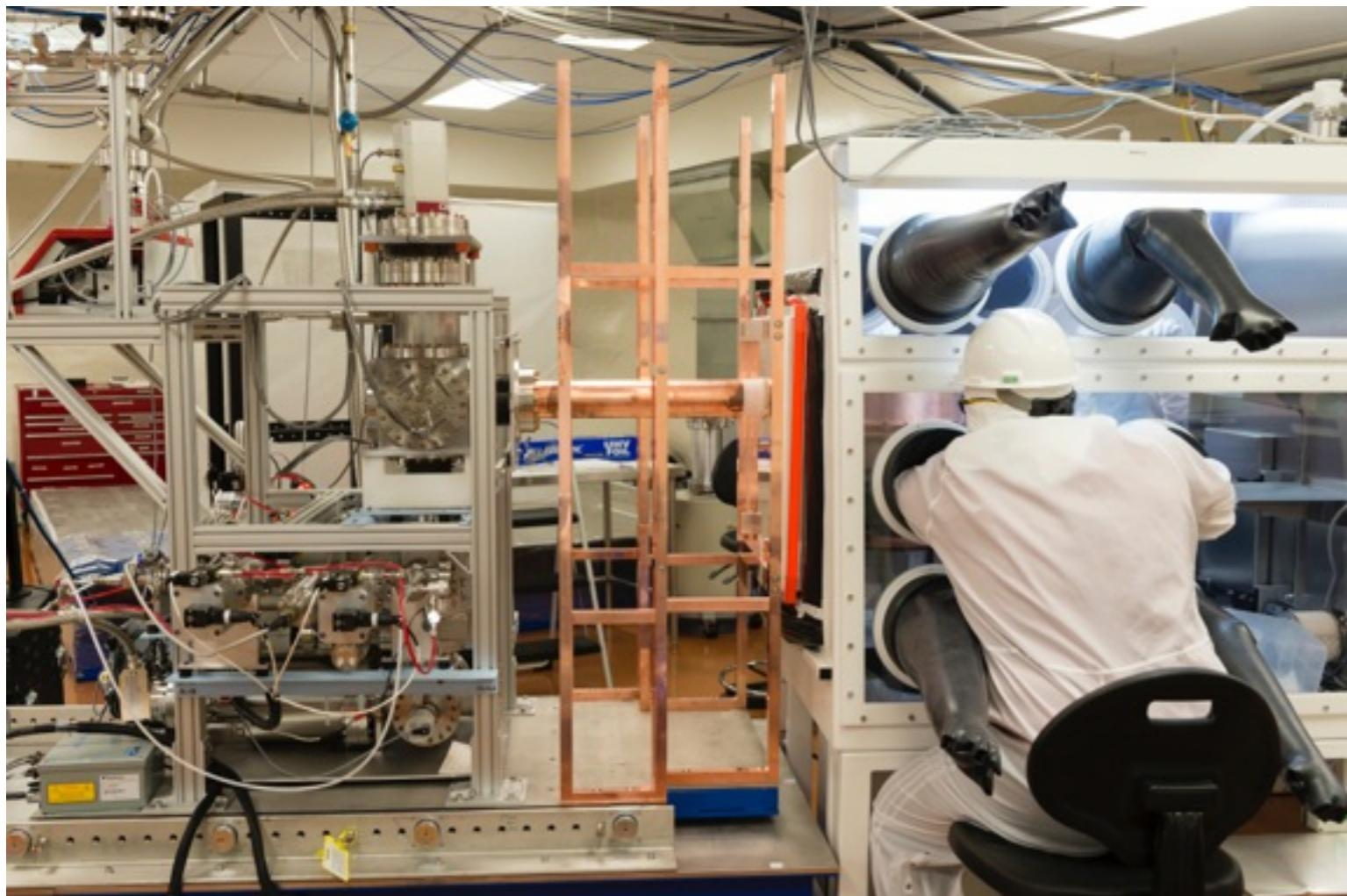
Prototype Cryostat with three installed strings
