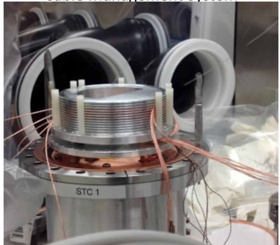
Loading string into string test cryostat in Glove Box
