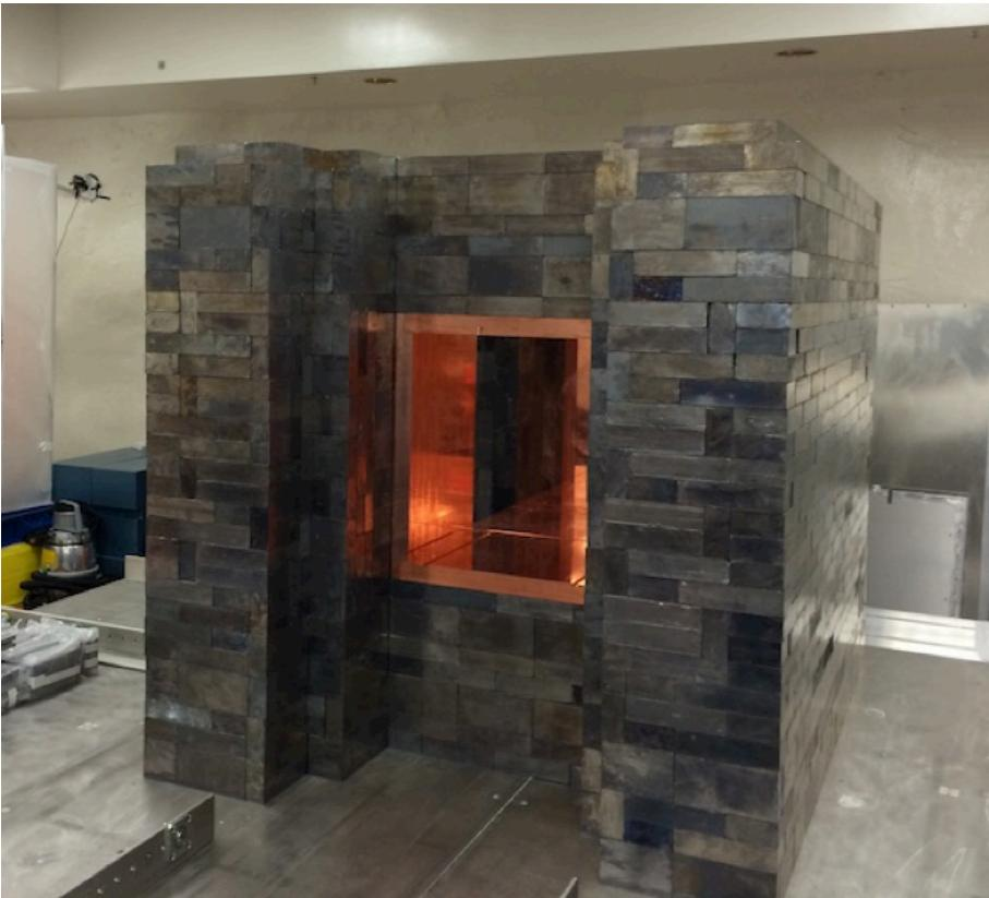
Shield with Radon exclusion box installed
