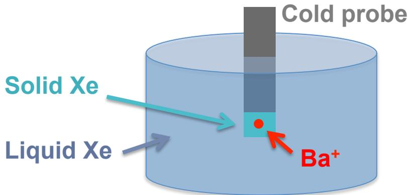
Detect single ion or atom on the probe with laser-induced fluorescence
