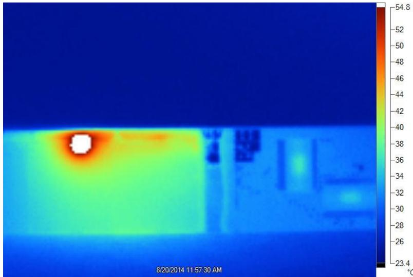
Post run IR picture showing a hot spot in digital section of a sensor. These hot spots are present on all ladders with increased current draw. Testing is still in progress.
