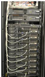
Cluster of 8 nodes of Fermi GPUs
