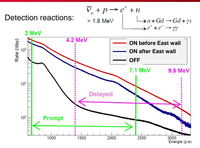
Reduction of the rate by 100/3 with the south/east wall shieldings
