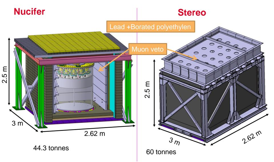
Heavy structure that should respect earthquake regulation of the installation
