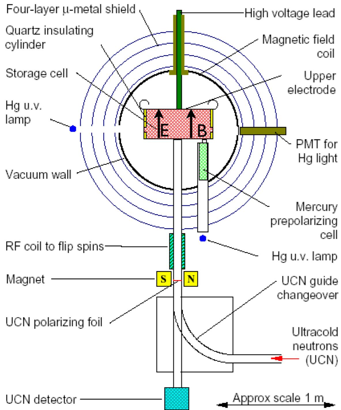
Ultra-cold Neutrons (UCN) in a storage cell (at  $T \sim 300$  K):  $\rho_{\text{UCN}} \sim 1/\text{cm}^3$
