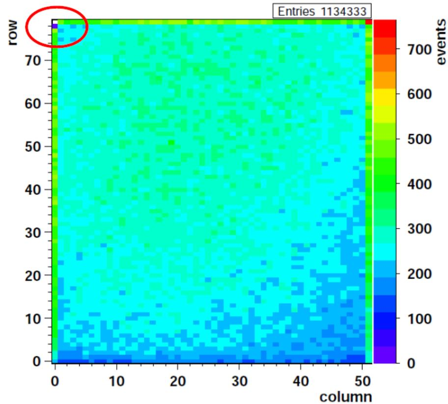
2 Missing bumps at top left corner (reconfirmed with beam profile in DESY test beam)
