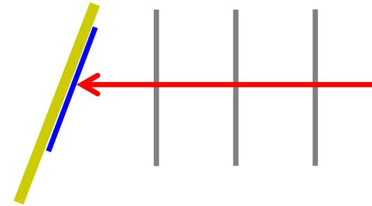
Position resolution calculated by comparing the track position interpolated by the telescope planes and the pixel hit position using **charge sharing** between rows
