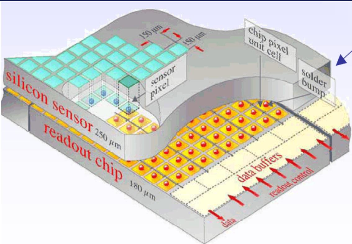
Silicon sensors with  $100 \times 150 \mu\text{m}^2$  pixels, bump bonded to CMOS readout chips for DC connection.
