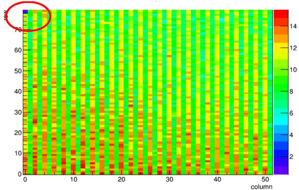
All pixels respond to test pulses – zero pulse height indicate missing bump
