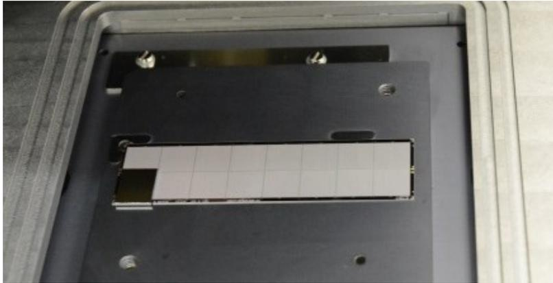
readout chip bonded onto the Si sensor with 160 N force @ 240°C
