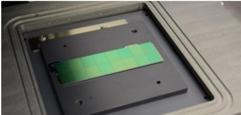
In-situ solder reflow performed in formic acid atmosphere
