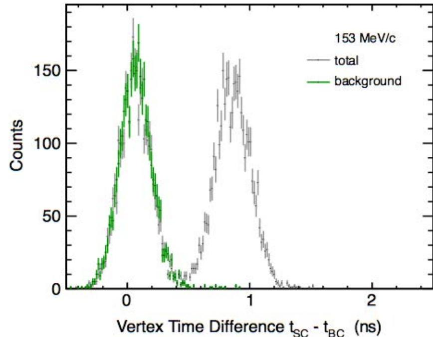
In situ measurement of muon decay-in-flight background from events upstream & downstream of the target.
