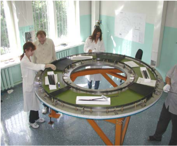
Installation of straws (tests leak tightness)
