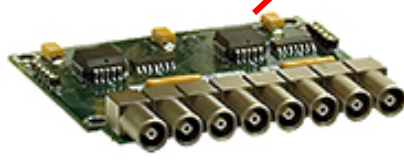
8 NIM/TTL in/out channels
