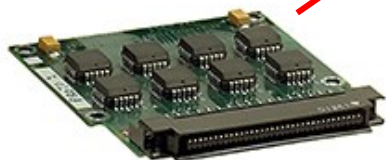
32x LVDS/ECL input channels
