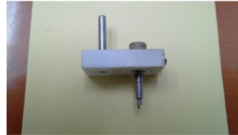
Inserted an Hypodermic needle in the suction nozzle
