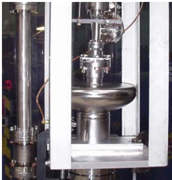
Figure 8: The half-cell cavity with plug. Test results with and without the lead coating.
