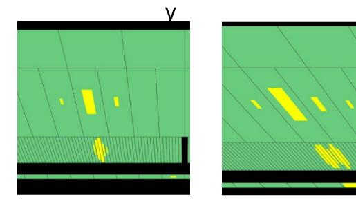
•Width of cluster allows to separate photons from hadronic jets •Substructure of shower using the finely segmented first calorimeter layer allows to separate photons from hadronic jets with leading  $\pi^0$
