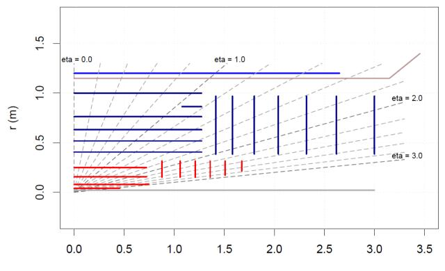
z (m) Upgraded Strip Tracker Layout > 5 +1 barrel layers D > 7 endcap layers
