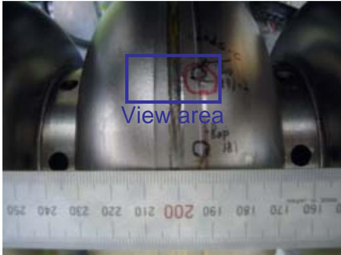
Twin spots were observed on the heat-affected zone (HAZ). EBW seams were very smooth at all cells equator.
