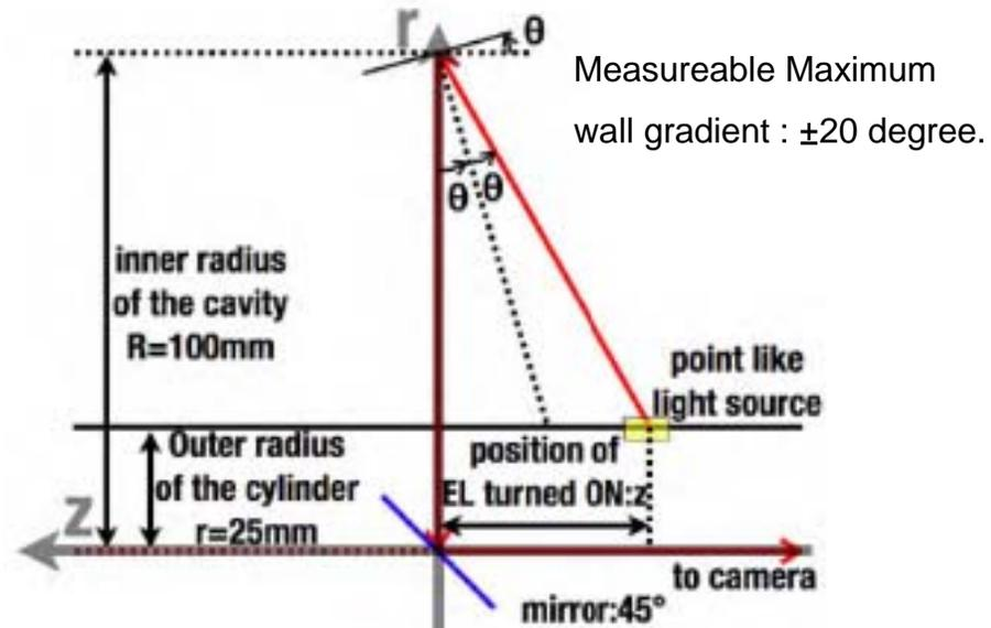
Schematic drawing of the wall gradient measurement
