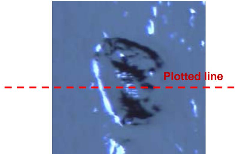
STF Baseline #5 cavity after EP-1 (125 $\mu\text{m}$  removed)
