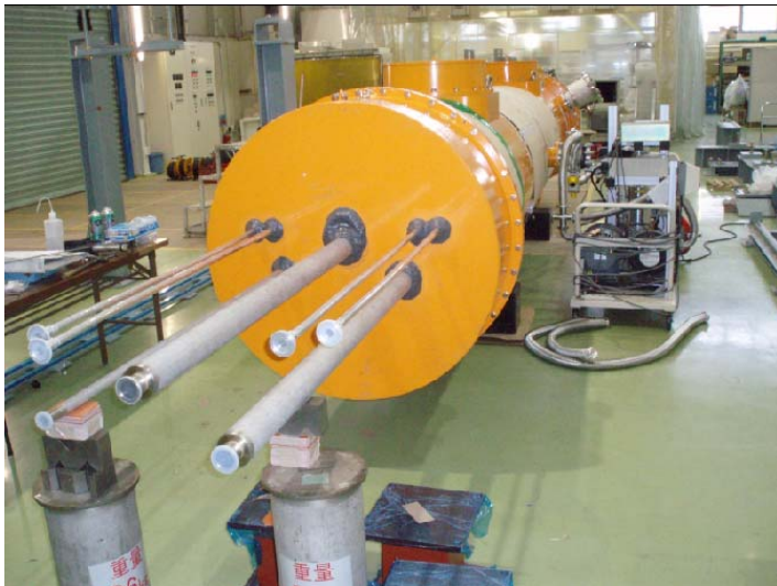
For the leak test, the vacuum vessel was closed with special end caps.
