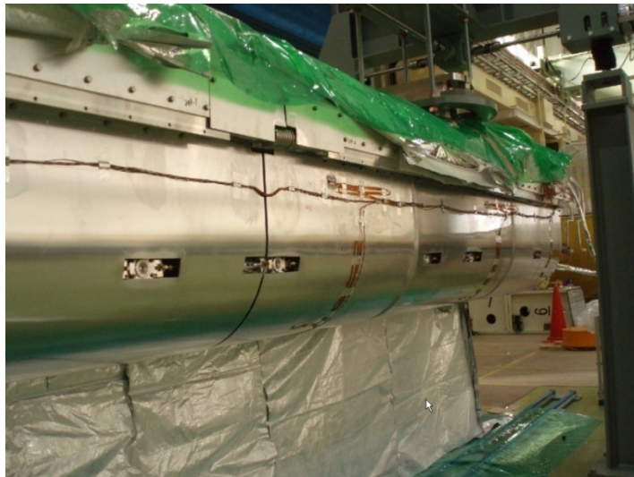
Setting the temperature sensors and signal wires. Checking the sensors. Wrapping SI over the thermal shields.
