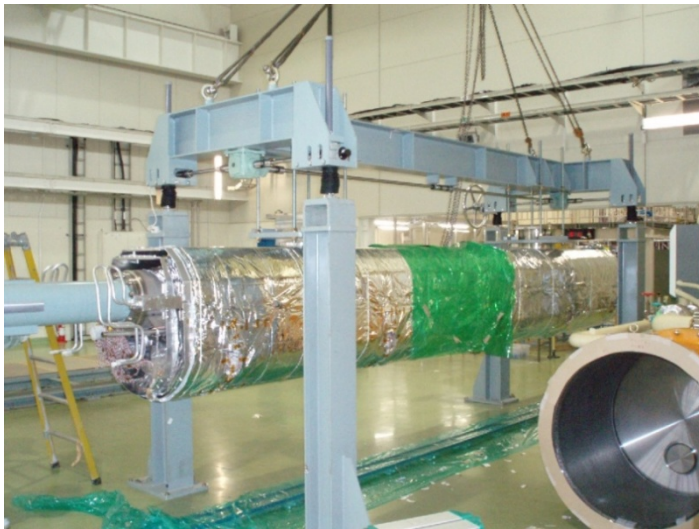
Hanging the cold mass with the upper-side of the assembly trestle.
