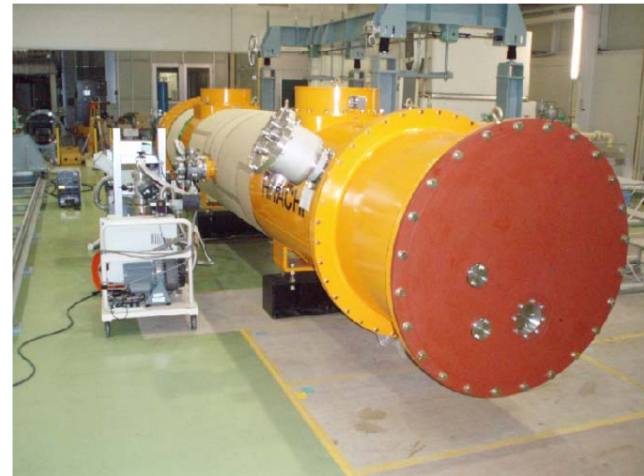
Final leak test in the assembly area. The vessel was in a vacuum condition, and the cooling pipes were pressurized with helium gas.
