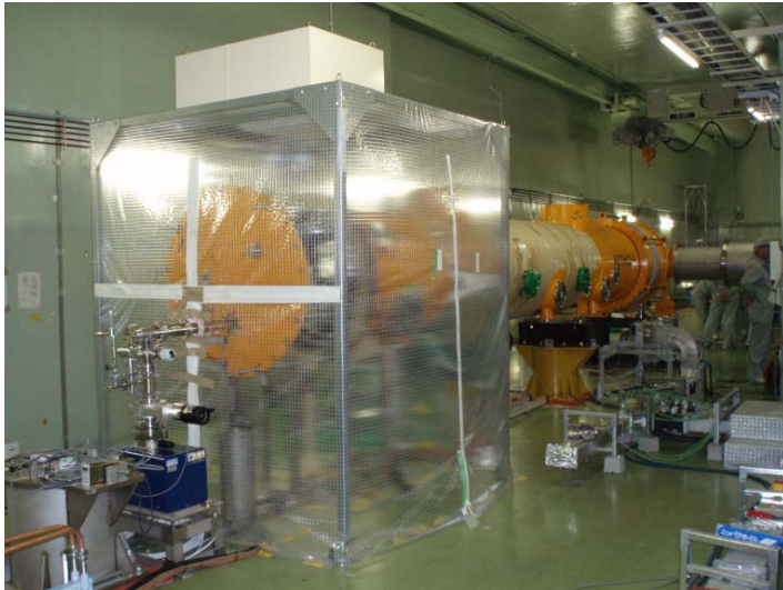
Assembling the beam pipe in the local clean room. Leak test was done after the assembly.
