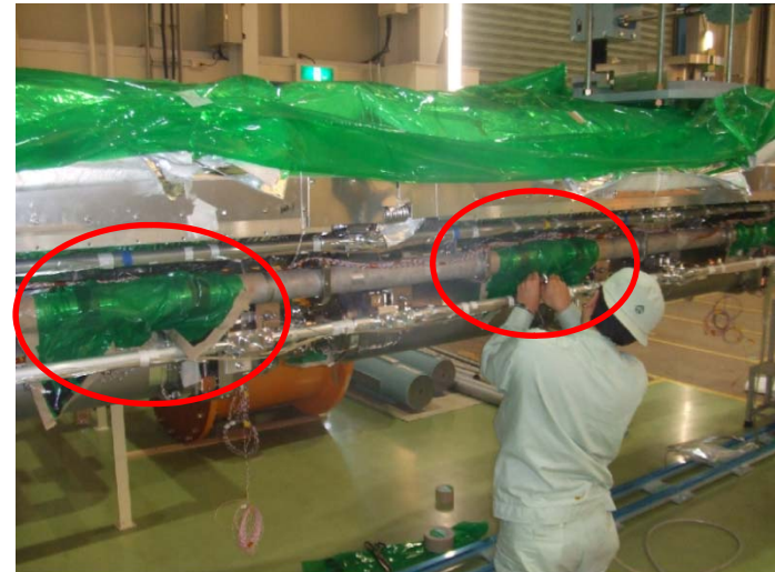
Leak test of cooling pipes. Masking the test parts.
