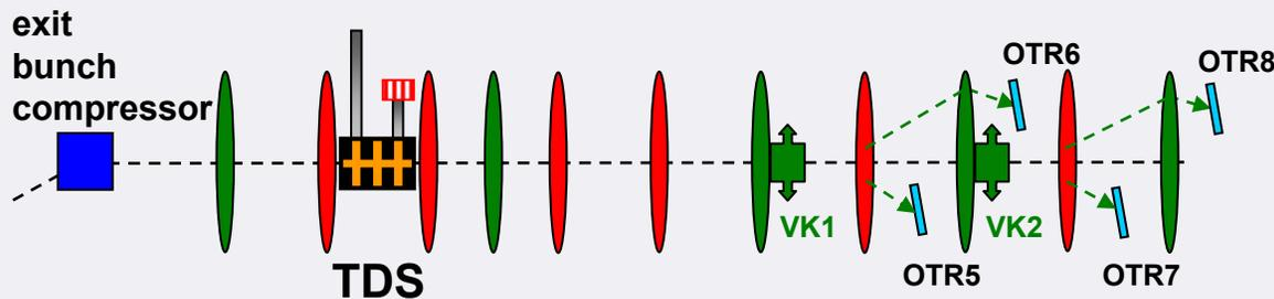
XFEL layout: Single bunches can be extracted from bunch train  $\rightarrow$  continuous monitoring of bunch slice parameters
