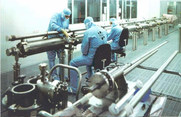
Using experience gained at DESY and results of industrial studies, the assembly facility for all 100 XFEL modules will be set up at the CEA-Saclay site.
