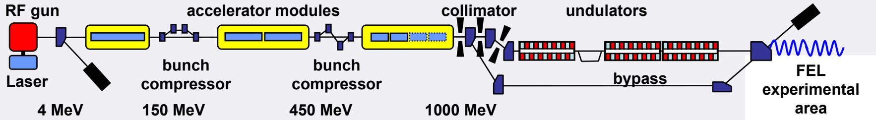
→ **6 accelerator modules** routinely in operation; design beam energy & photon wavelength (6.5 nm) since Oct. 2007
