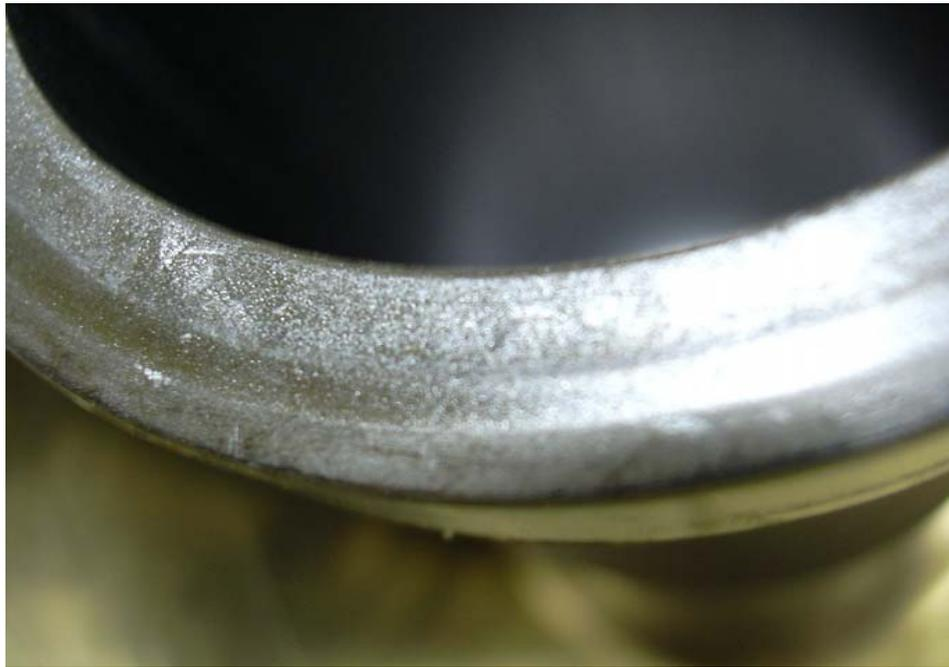
Some 50 cold warm cycles and some 10 mounting dismounting procedures later: Gasket imprint on the flange, 0,16 mm deep, resulting in cold leaks
