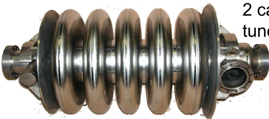
2 cavities with tank, tuner, inner mag shield
