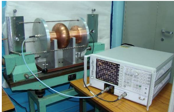
Bead-pull measurement set-up for an assembled cavity
