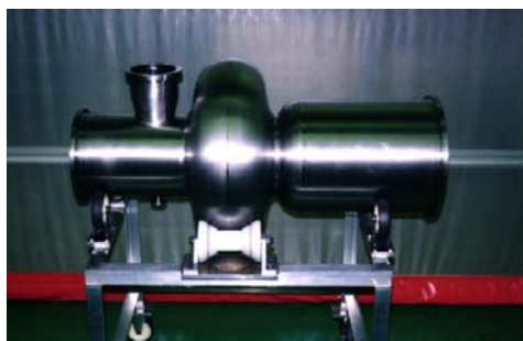
509 MHz Nb single-cell cavity. Large iris dia. of 220 mm with a cylindrical BP of 300 mm in dia.
