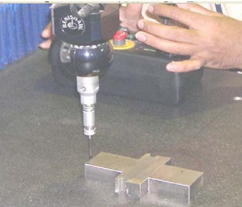
Distortion measurement(on CMM)
