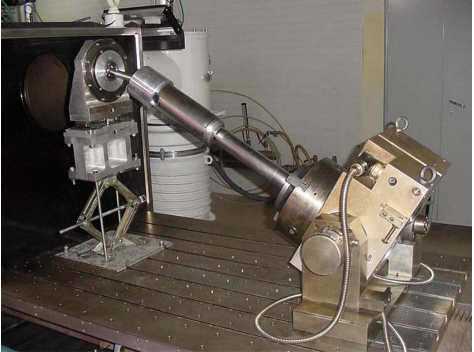
Electron Beam Welding of Nb Central Conductor
