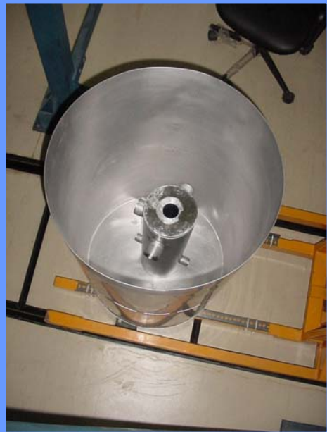
Resonator inside Nb getter box before annealing
