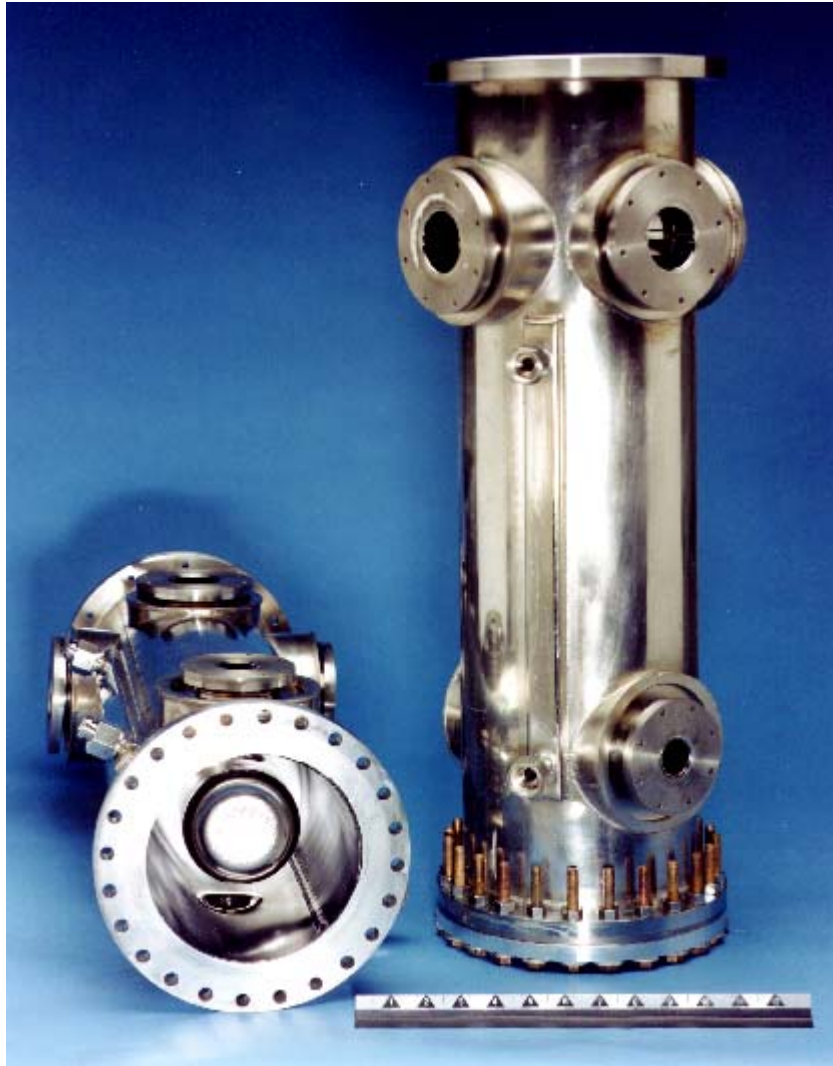
IUAC Quarter Wave Resonator (QWR)
