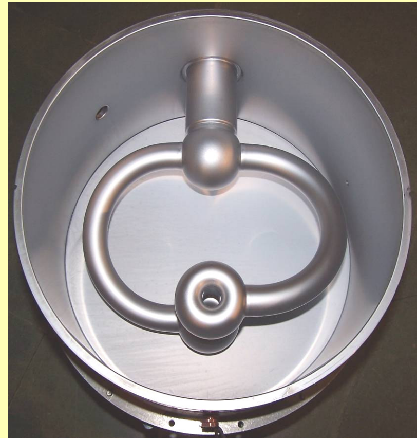
After Lead Plating
