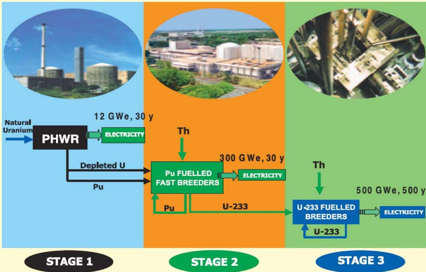
Kalpakkam has the unique distinction of being the only place in the world, where all the three fissile isotopes viz., U-235 [MAPS], Pu-239 [FBTR] & U-233 [KAMINI] are used as fuel in reactors.
