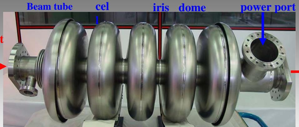
Superconducting cavity (IPN Orsay) – 5 cells, 700 MHz,  $\beta=0.65$
