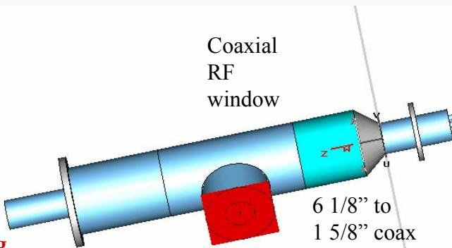
Adjustable  $\lambda/4$  shorted stub in coaxial configuration (6 1/8")
