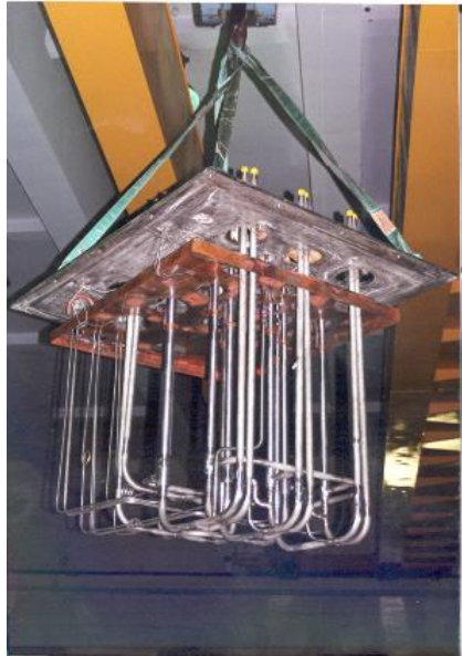
VALVE BOX AFTER ALL WELDING, THEMAL SHOCKING, AND LEAK TESTING
