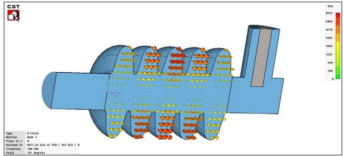
Magnetic field lines inside the cavities
