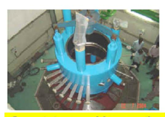
Cryostat assembly over the magnet
