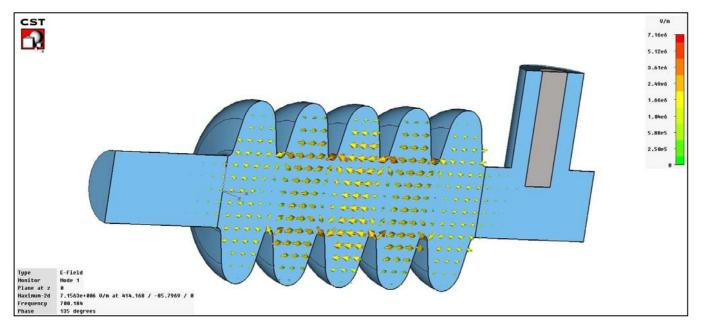
Electric field lines inside the cavities
