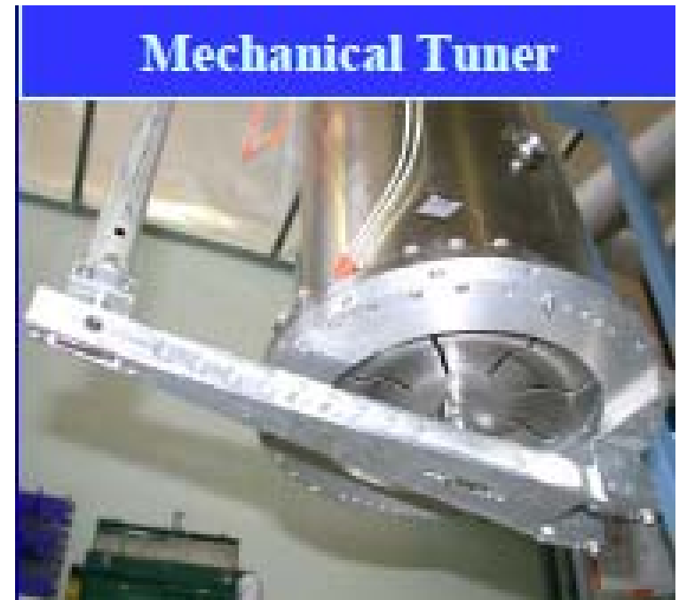
Bulk Nb slotted tuning plate (in a protective plastic bag).
