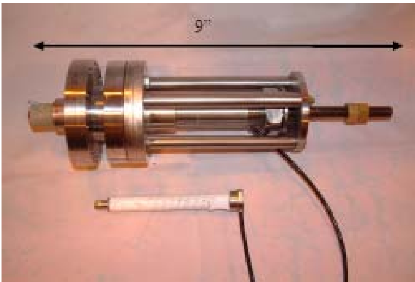
piezoelectric fast tuner guide assembly (above) and bare piezoelectric stack
