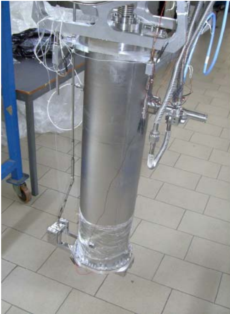
Low- \beta cavity equipped with new tuner and cooled coupler, ALPI
