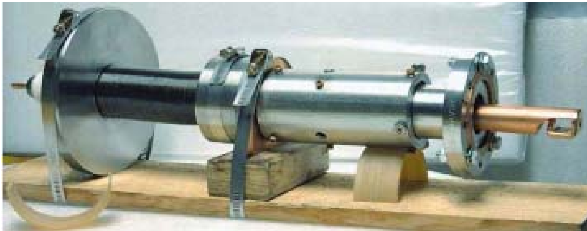
cw inductive power coupler – ANL for spoke cavity Fully variable over 50 dB
