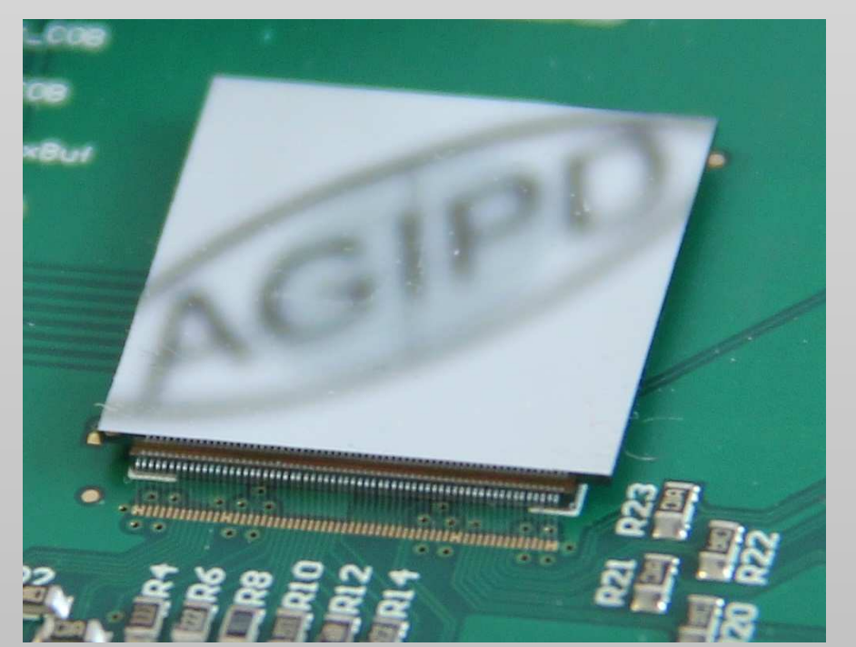
AGIPD1.0 single chip assembly
