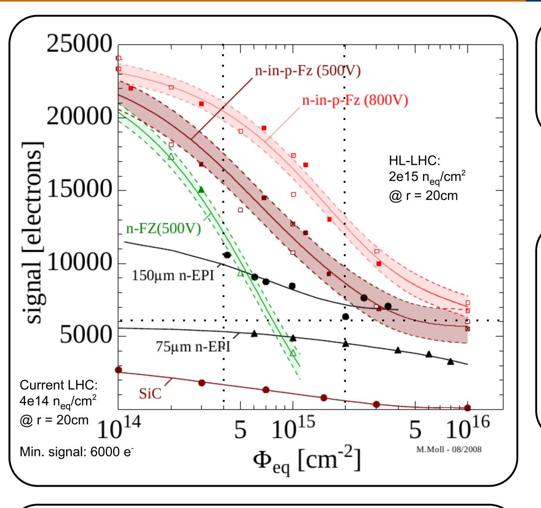
High Luminosity-LHC from 2023:  $\rightarrow$  Increase luminosity by a factor of 5  $\rightarrow$  Even harsher radiation environment
