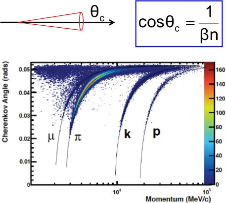
2 RICH detectors with 3 different radiators ensures good PID over full momentum range.
