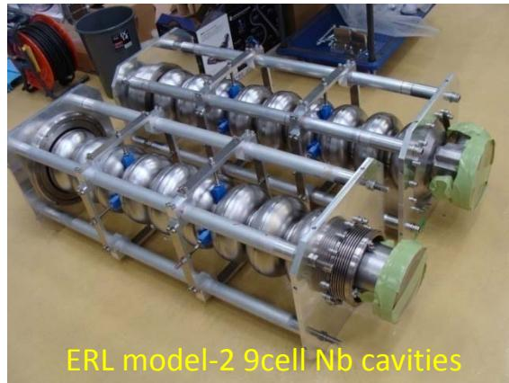
**9cell superconducting cavity**
