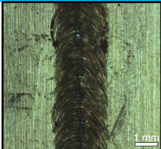
Equator EB welding (Cu cavity)
