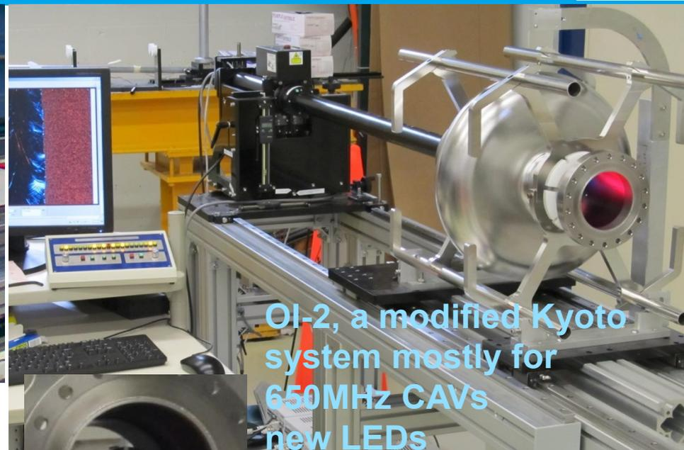
**OI-2, a modified Kyoto system mostly for 650MHz CAVs new LEDs**
