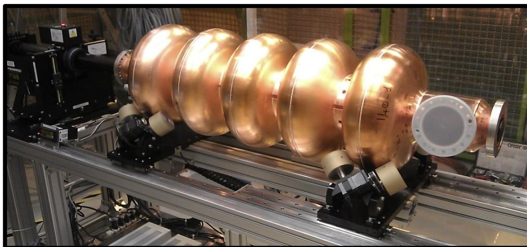
SPL copper mock up on the bench for the first test
