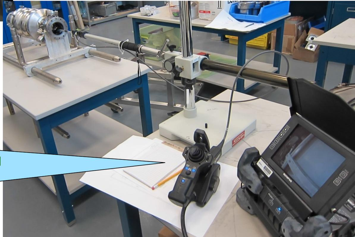
Optical system based on a **mirror** and **microscope camera** connected to a computer
