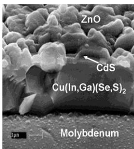
Fig.1: Cross section SEM of a chalcopyrite solar cell
