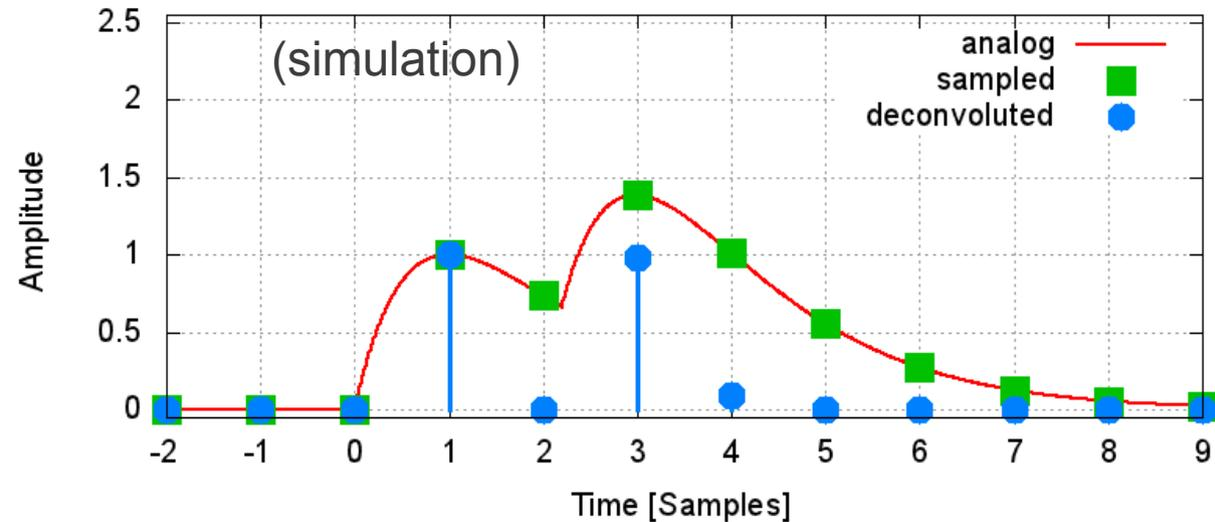
Time reconstruction performance ( $T_{smp} = T_{peak} = 60$  ns)
