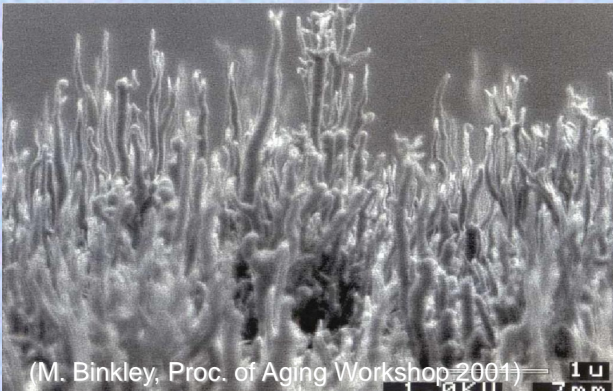
Unprocessed gas from the new vendor: 1400 ppm ethylene, 1100 ppm propylene, 600 ppm propane. Wire aged to 30% gain loss (about 0.13 coulomb/cm).
