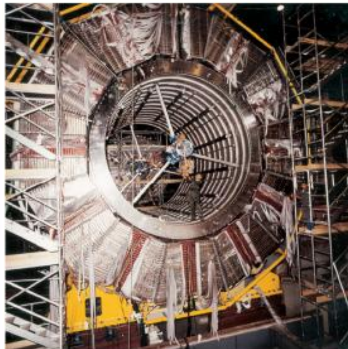
Hall probe measuring device being set up in the coil.
