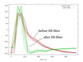
$CSA \rightarrow ADC \rightarrow IIR \ Filter \rightarrow \ hit \ logic \rightarrow \ message \ building \ \checkmark$
