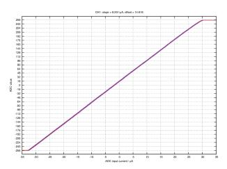
ADC curve: taken at 20 MHz sample rate, preliminary bias settings
