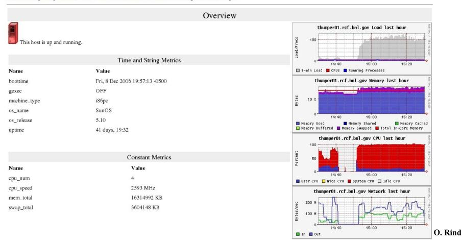
Test 6: 75 clients sequentially writing 3x1.5GB files (green line) + 75 clients sequentially reading 4x1.5G randomly selected files (blue line)
