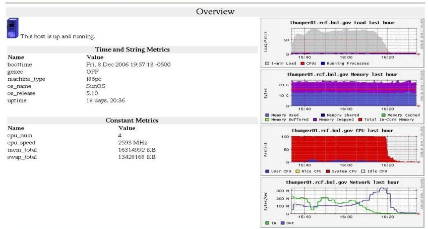
Test 5: 75 clients sequentially writing 3x1.5G files (green line) + 75 clients sequentially reading 4x1.5G randomly selected files (blue line) @ 250-300MB/sec.
