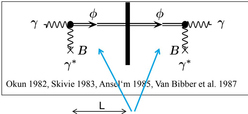
Coherent production and regeneration:  $P_{\gamma \rightarrow \phi} \propto (B \cdot L)^2$
