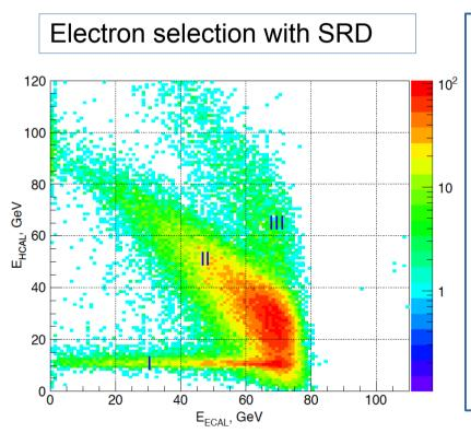
Region I —> rare QED dimuon production e- Z  $\rightarrow$  e-Z $\gamma$ ;  $\gamma \rightarrow \mu + \mu$ -, characterised by the energy of  $\approx 10$ GeV deposited by the dimuon pair in the HCAL.  $\rightarrow$  benchmark for the MC and estimate systematics in signal reconstruction.
