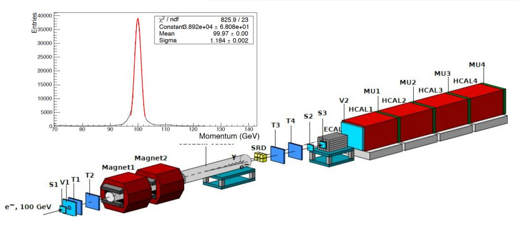
The magnetic spectrometer → Reconstruction of the incoming particle momentum
