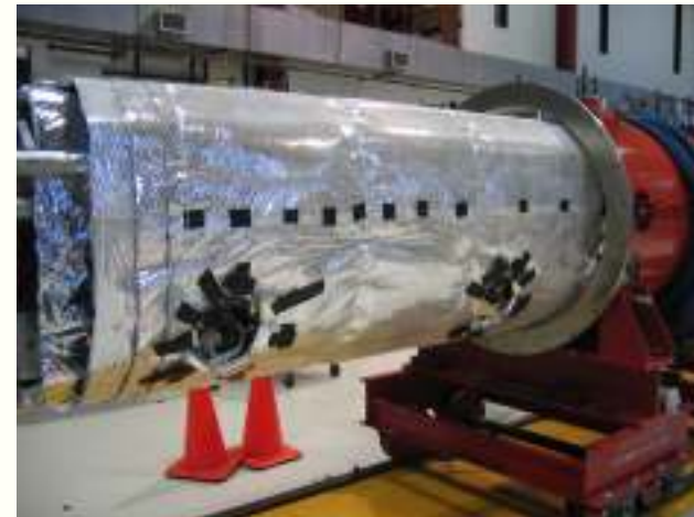
Cold Mass to the Vacuum Vessel assembly
