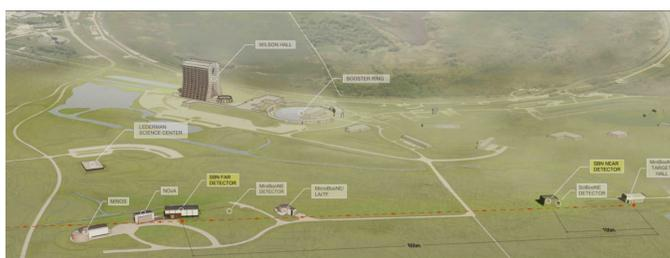
The Short-Baseline Program at Fermilab will probe oscillation anomalies and measure precision neutrino-argon cross sections (GeV range), using three liquid argon time projection chambers along the Booster Neutrino Beam.<sup>[2]</sup>
