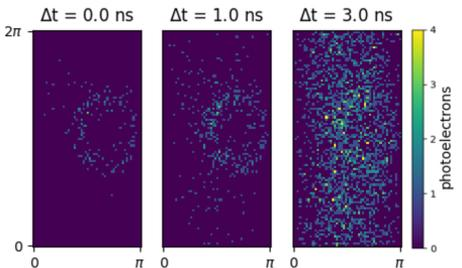
KamLAND-Zen, the leading LS detector has time resolution  $\sim 1.5\text{ns}$ ; NuDot [1] will have time resolution  $< 200\text{ps}$ .
